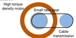
Fig. 1. Quasi-direct drive actuation using high torque density motor and low ratio transmission has advantages of reduced mass and high-backdrivability. Combining with the cable transmission structure, our hybrid soft exoskeleton design using quasi-direct drive actuation attempts to minimize mechanical impedance to human movement.
