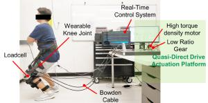
Fig. 2. A healthy subject performs squatting with the hybrid soft exoskeleton that uses soft cable transmission with rigid customized wearable structure. The quasi-direct drive actuation consisting of high torque density motors and low transmission ratio gears makes the exoskeleton lightweight and highly-backdrivable.
